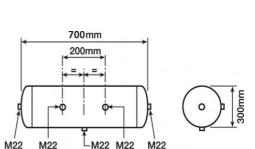
45LTR AIR TANK 300mm x 730mm LG U-BOLT MOUNTED SA1317
