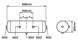
60LTR AIR TANK 300mm x 920mm LG U-BOLT MOUNTED SA1301 £84.01
